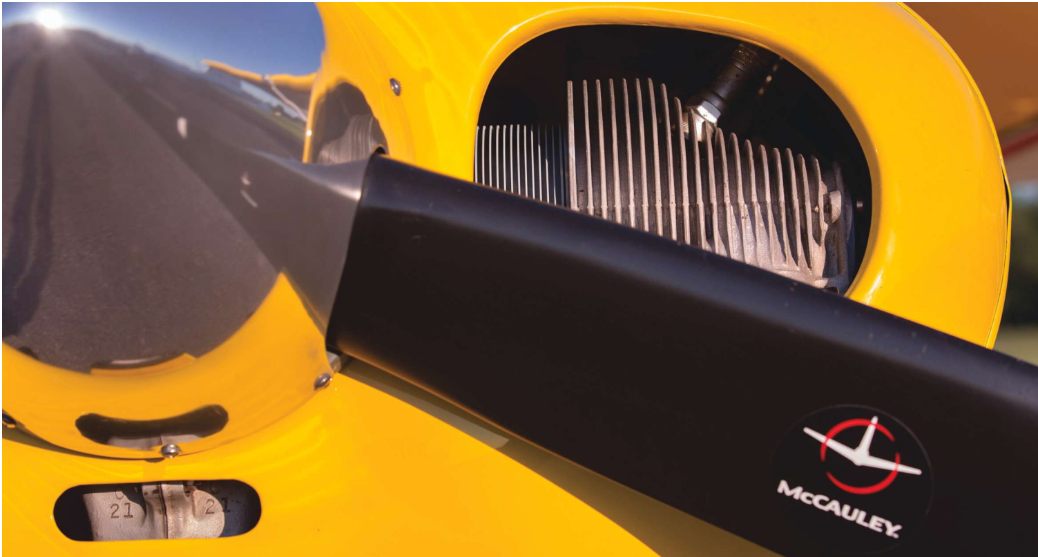
The Continental C-90 engine helps the airplane perform nicely, even with two people on board.
