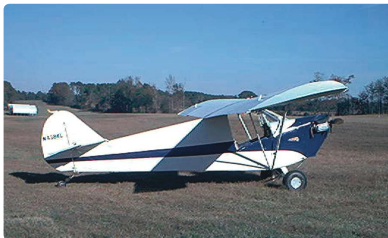
The Headwind in the photo above uses a spring gear and direct drive VW, while the Headwind below uses the rubber wafer damped gear. Its Maximizer-reduced VW has a higher thrust line, which produces the different nose profile.
