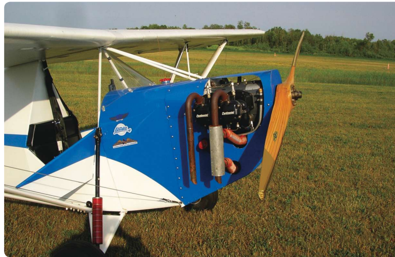
Landing shocks are absorbed by stacks of rubber wafers or Chevy motor mounts.
