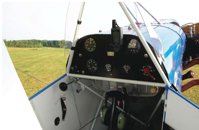
The cockpit can be built to fit almost any size pilot. The door can be eliminated.
