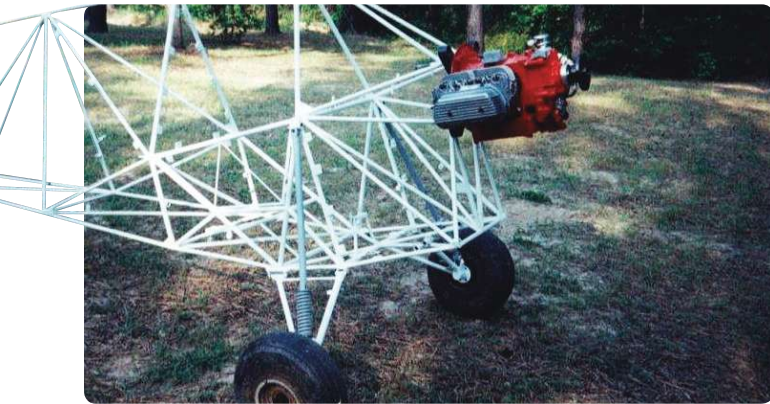
The fuselage structure features a triangular cross section with the top longeron running from the main wing fittings to the rudder post. The motor mount is integral to the fuselage.
