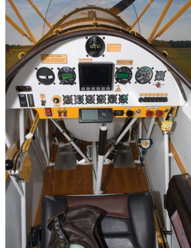
The captain's seat sports a Dynon primary flight display, but is otherwise spartan, as befits a craft intended for VFR, day-only flying.
