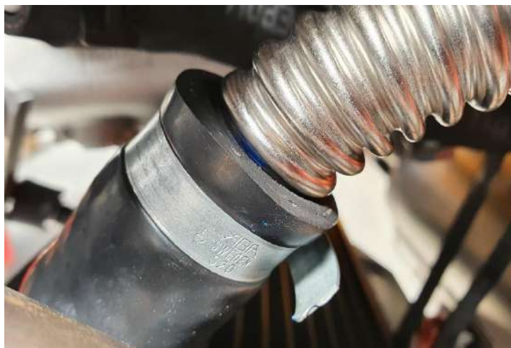
Figure 8: Water hose on corrugated pipe
