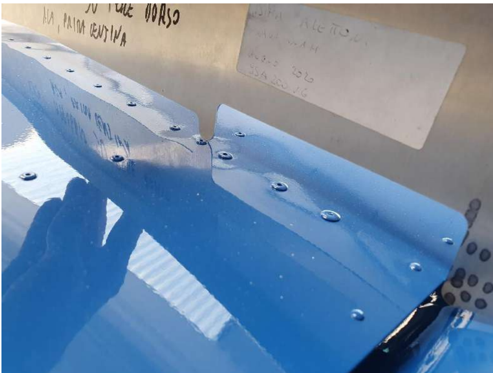
Figure 39: Position of jig SA200VG near the first rib rivets line, aligned to wing trailing edge
