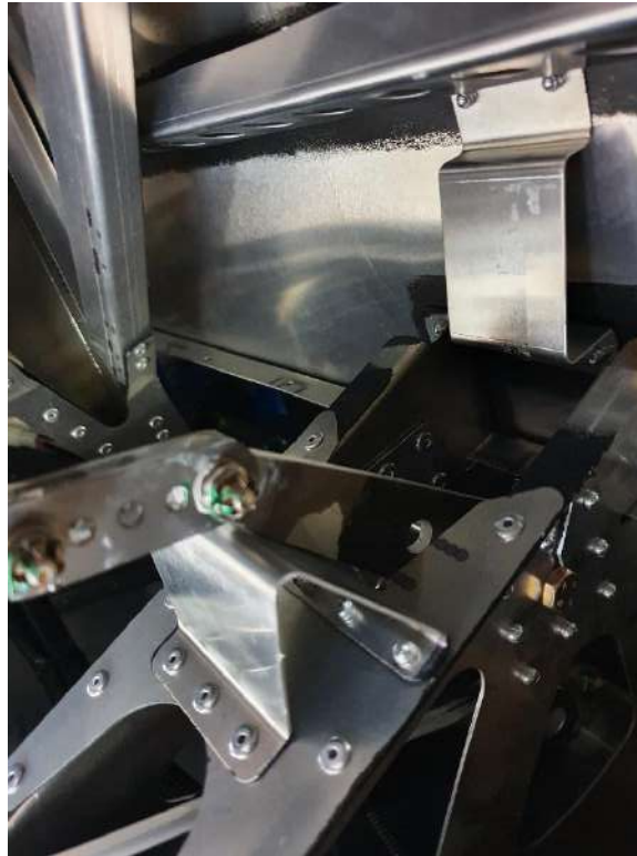
Figure 43: Longitudinal line bell crank on the full nose up position, against stop
