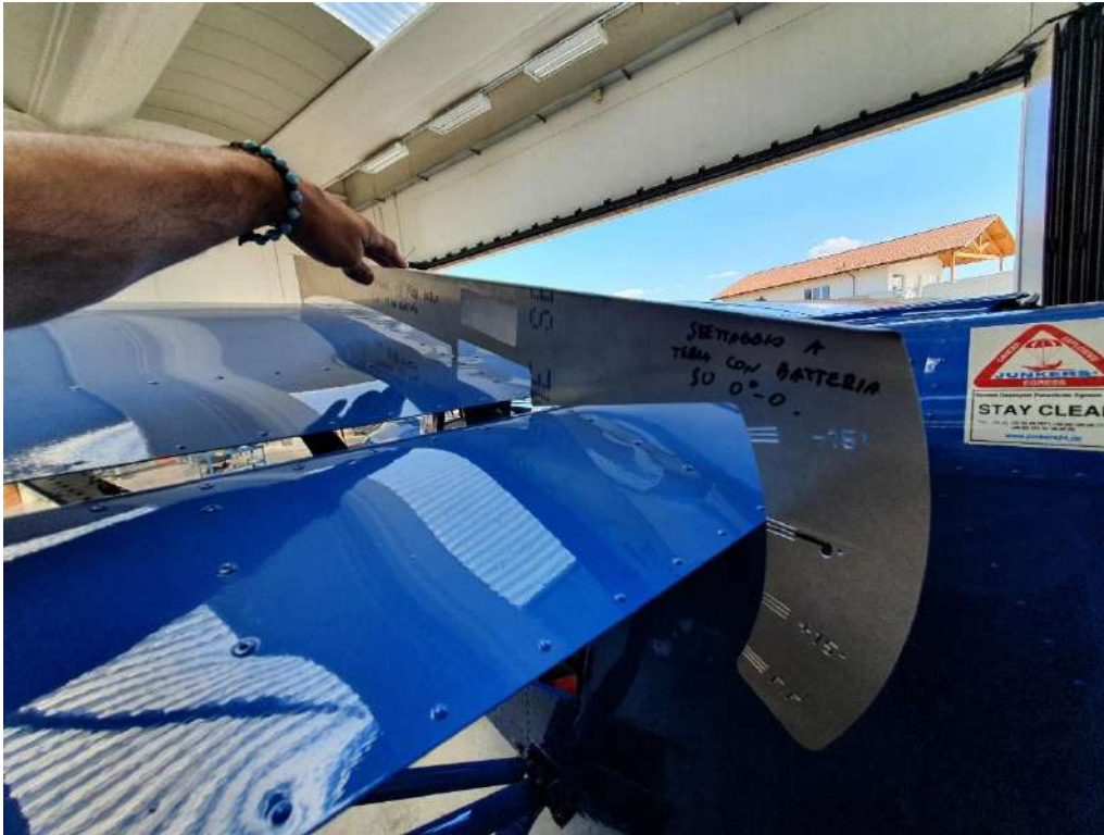
Figure 38: Flaperon jig SA200VG and position on the first wing rib
