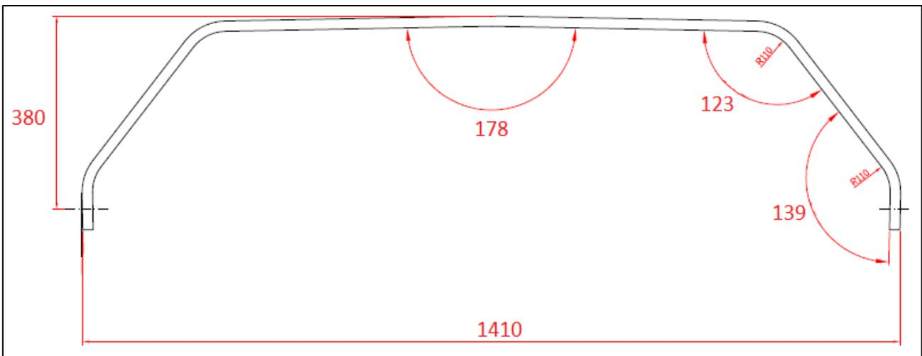
Figure 11: Main landing gear spring design nominal dimensions (unloaded)
