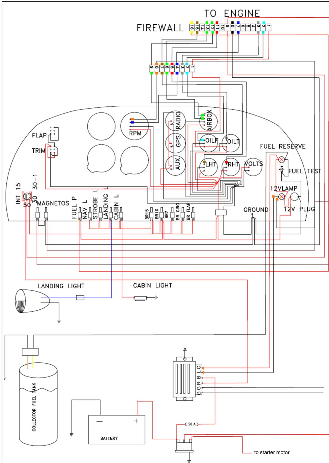
Figure 38: Electrical wiring firewall backward
