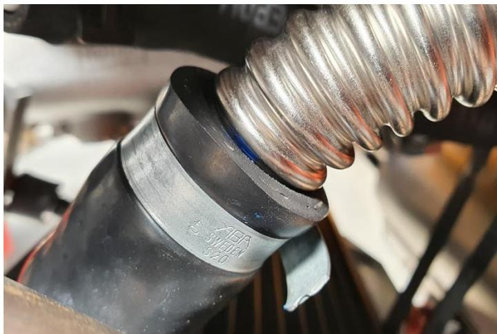
Figure 9: Water hose on corrugated pipe
