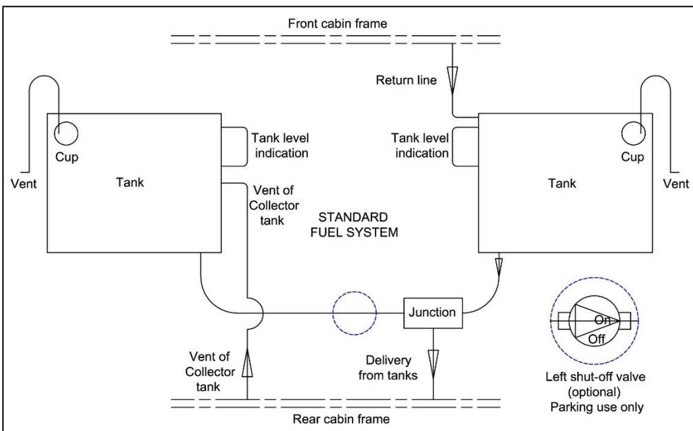
Figure 24: Wing standard fuel system
