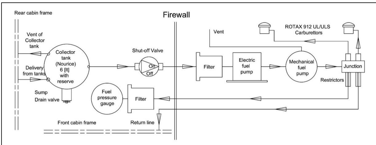
Figure 27: Fuselage and Rotax 912 UL/ULS fuel system
