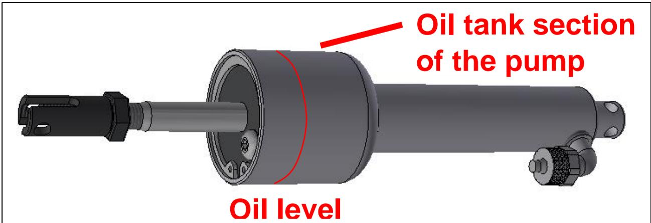
Figure 48: Brake pump (seen horizontally, not vertically like the airplane installation)
