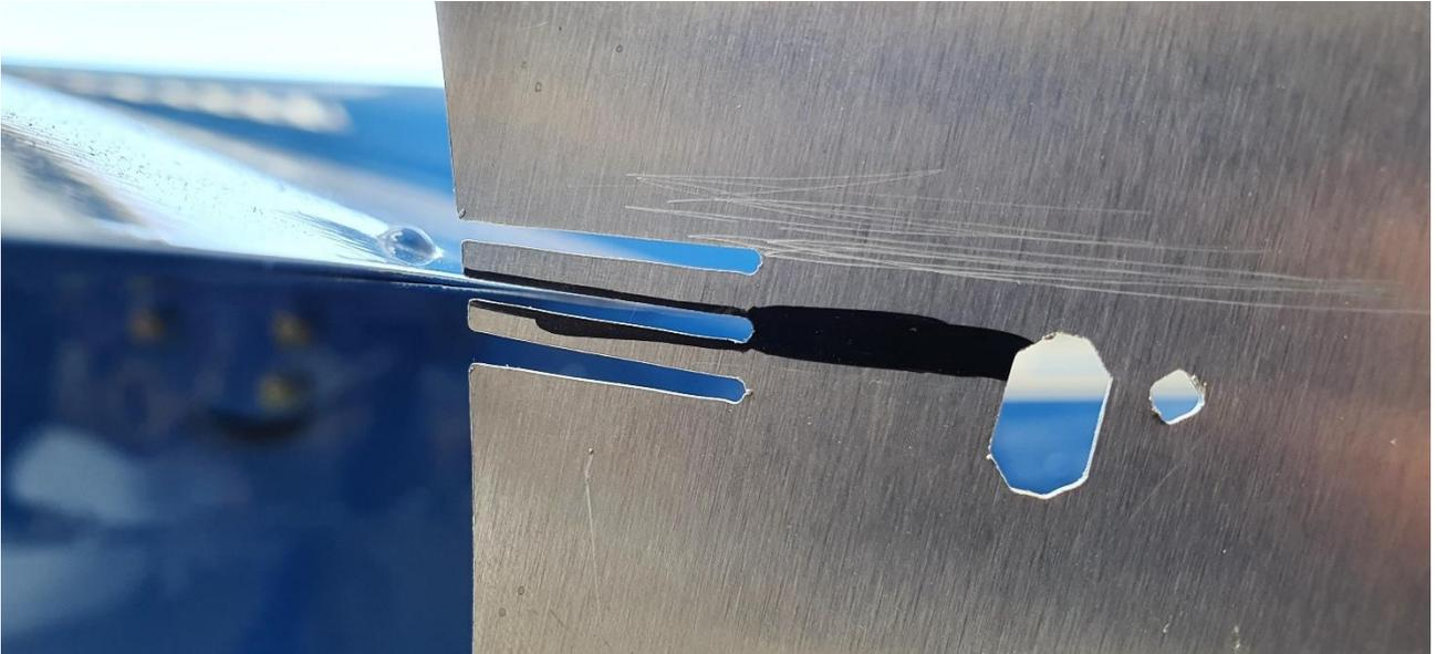
Figure 41: ZERO setting of the left inner Flaperon. Marks of +/- 0.5° of tolerance
