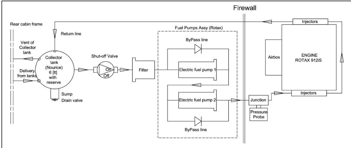
Figure 28: Fuselage Rotax 912 iS fuel system
