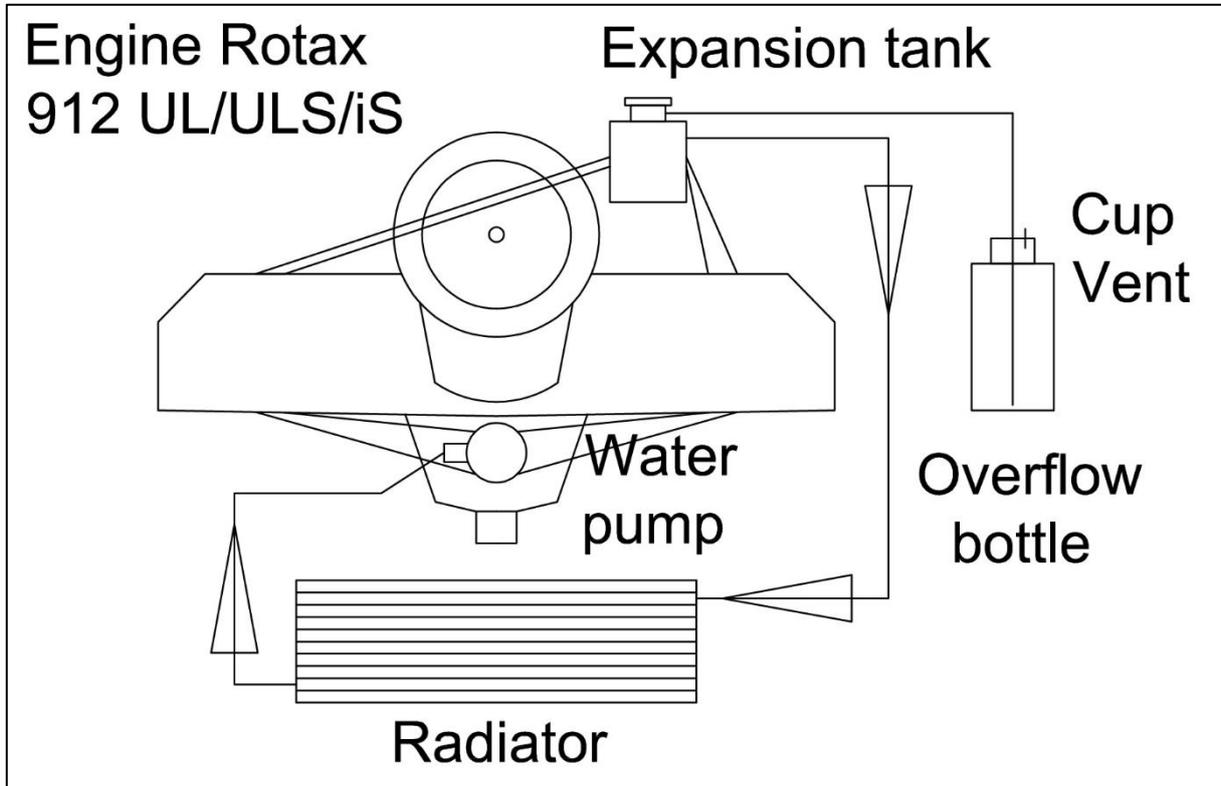
Figure 31: Rotax 912 UL/ULS/iS standard cooling system
