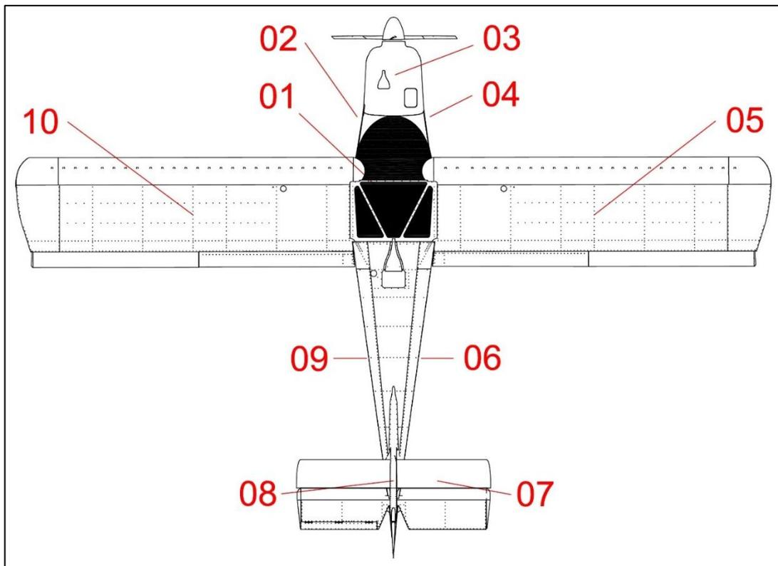
Figure 10: Daily pre-flight check sequence plan view
