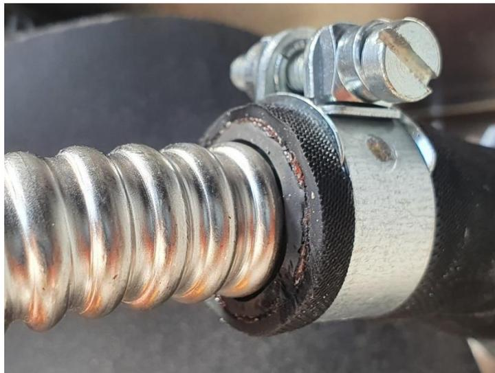
Figure 8: Oil hose on corrugated pipe
