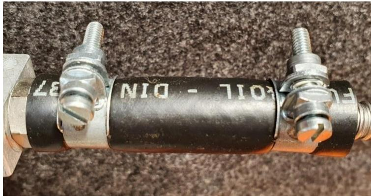
Figure 5: Fuel hose on fitting
