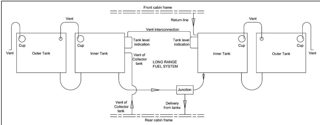
Figure 25: Wing double fuel tank system (interconnected tanks)
