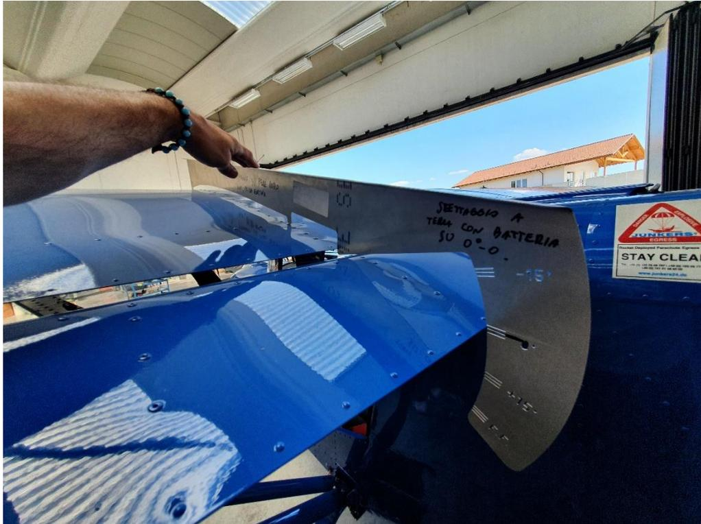
Figure 39: Flaperon jig SA200VG and position on the first wing rib
