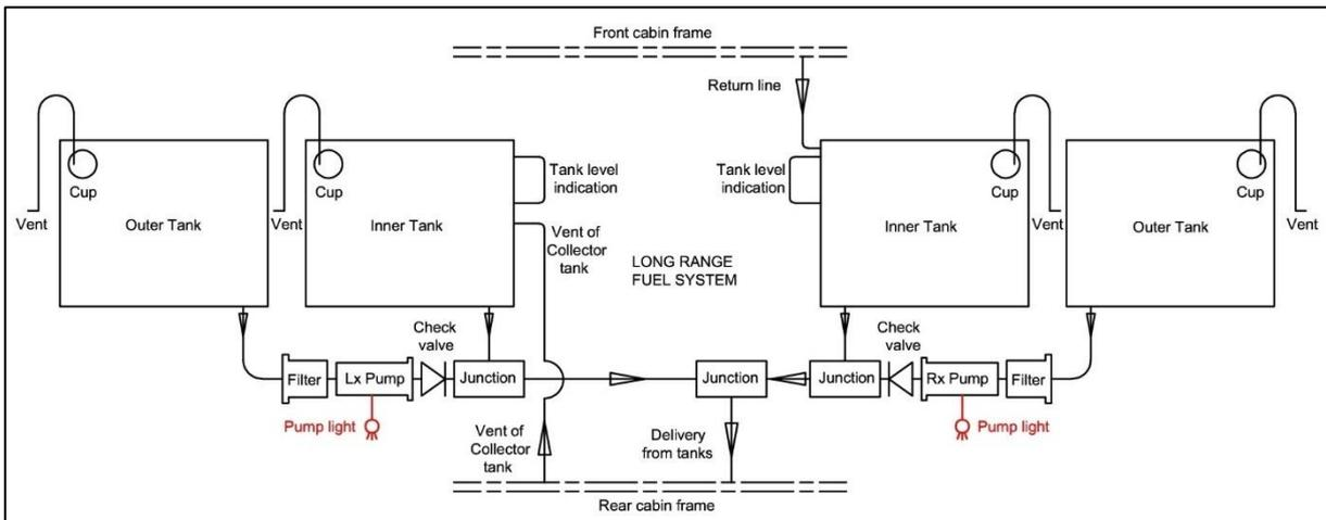
Figure 26: Wing double fuel tank system with transfer pumps
