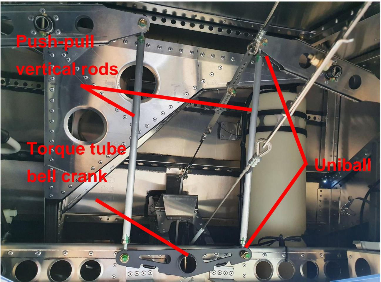
Figure 42: Push-pull rods for Flaperon setup
