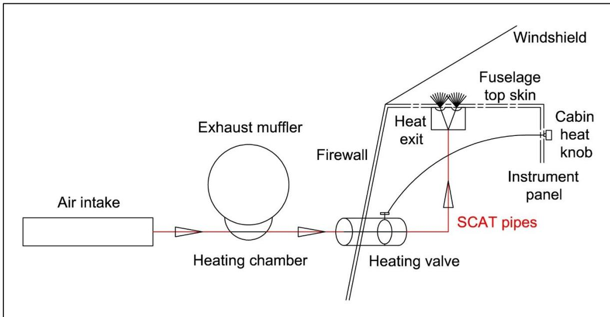
Figure 36: Cabin heating system
