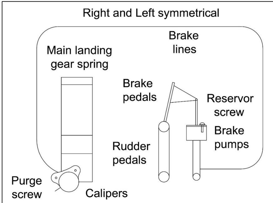
Figure 33: Standard brake system (only right side is shown, the left is identical, symmetrical)
