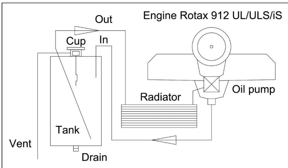
Figure 29: Rotax 912 UL/ULS/iS standard oil system
