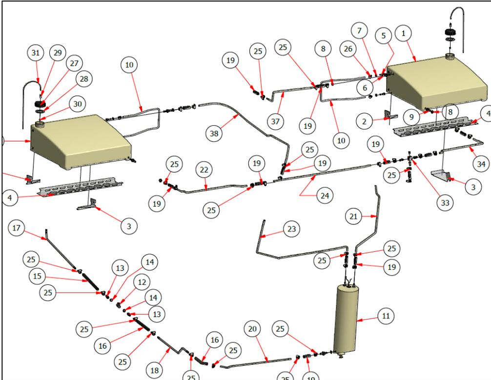
Figure 23: Airframe fuel system parts
