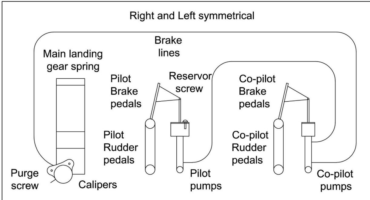
Figure 35: Double side brake system (only right side is shown, the left is identical, symmetrical)
