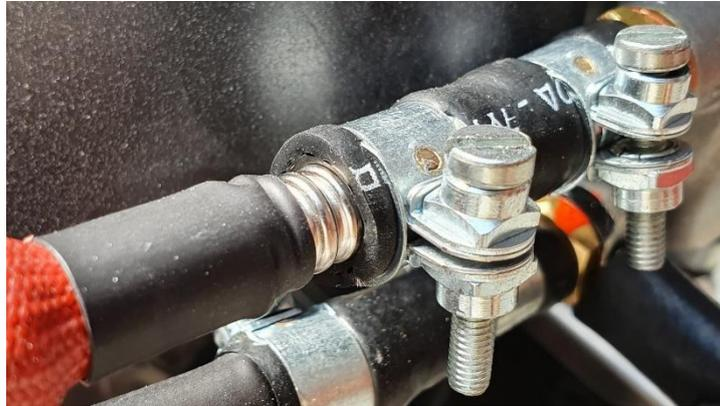
Figure 7: Fuel hose on corrugated pipe
