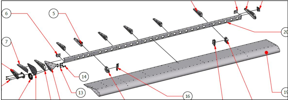
Figure 16: Left inboard flaperon
