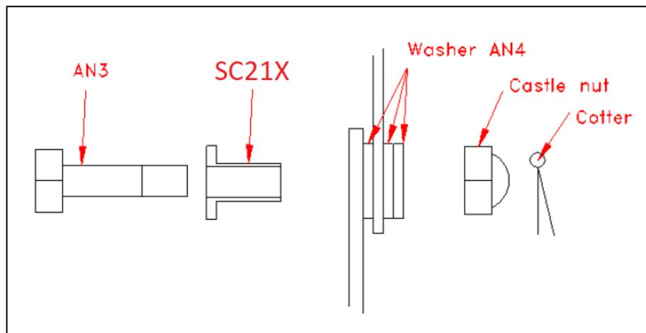
Figure 47: Control surfaces hinges
