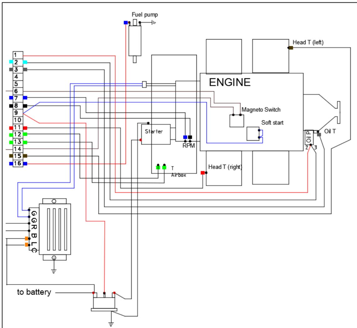
Figure 37: Electrical wiring of engine compartment
