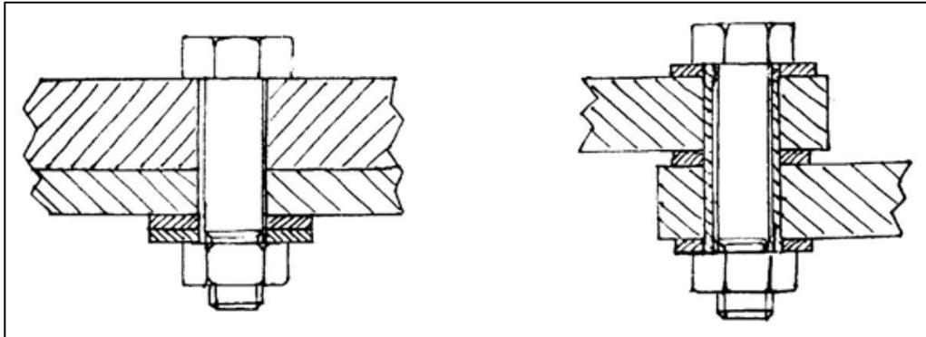
Figure 3: Threaded fasteners
