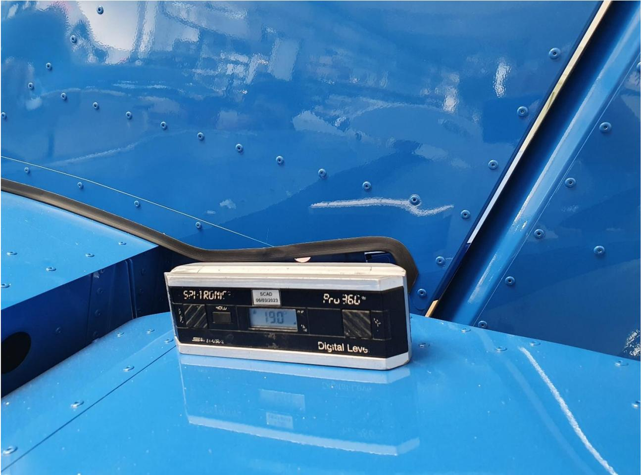
Figure 46: Elevator final setup deflection angle
