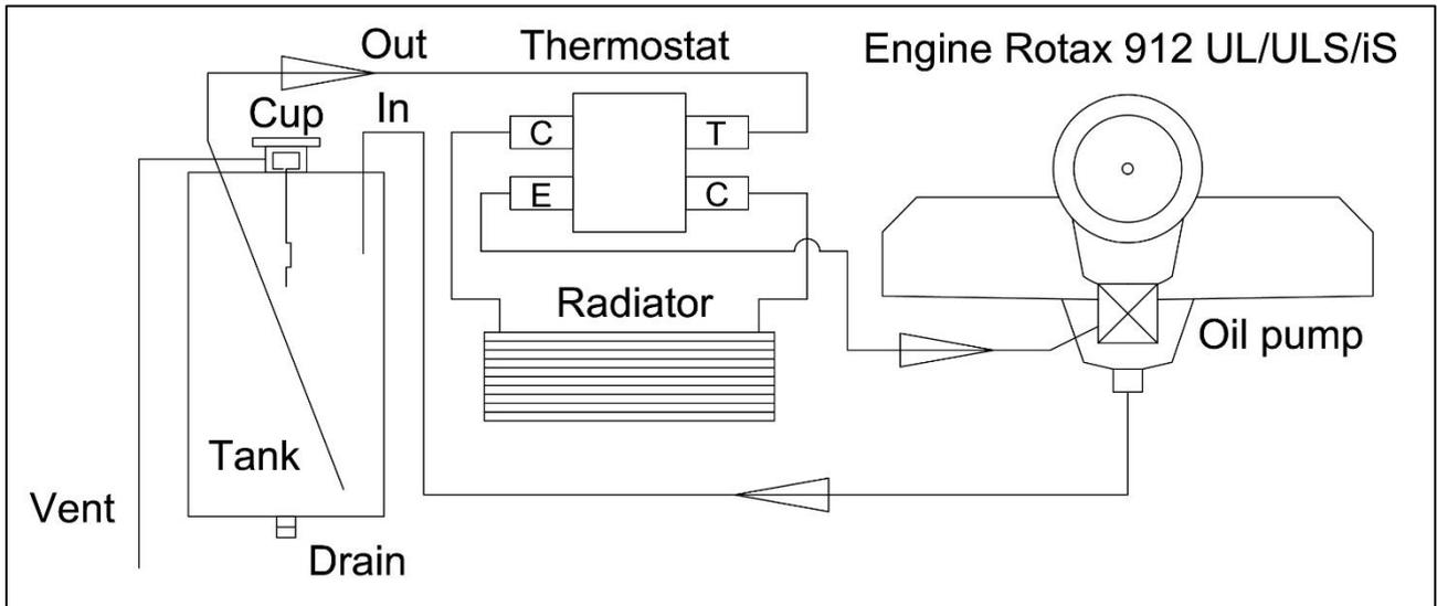
Figure 30: Rotax 912 UL/ULS/iS oil system with thermostat
