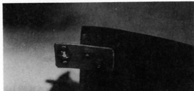
Photo No. 94: Cowl bracket for cam lock nut plate.
