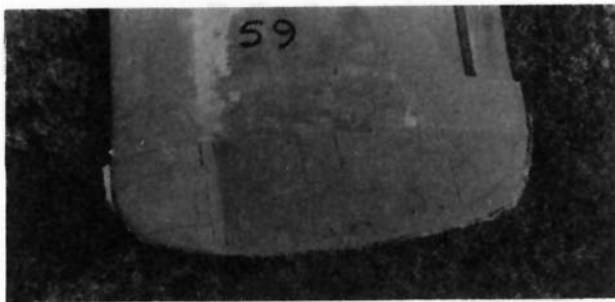
Photo No. 59: Foam in wing tip. Note the piece in line with front spar.
