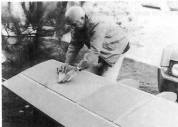
Photo No. 31: Rough sanding ribs down to top plates.
