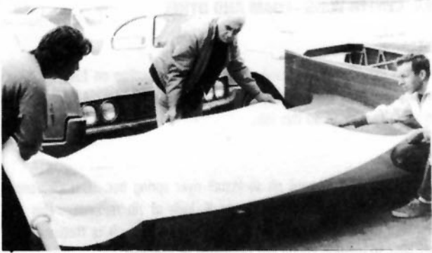
Photo No. 32: Laying out the Dynel to fit top of wing.
