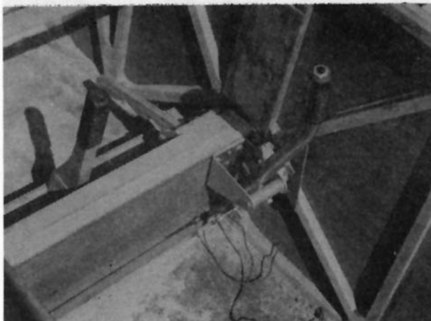
Side mounted control stick installed.
