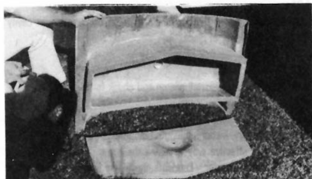
Photo No. 50: Tank bottom. Sump worked into bottom foam.
