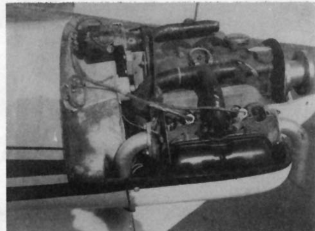
Engine compartment with top cowl removed; note upper engine mounts and magneto.
