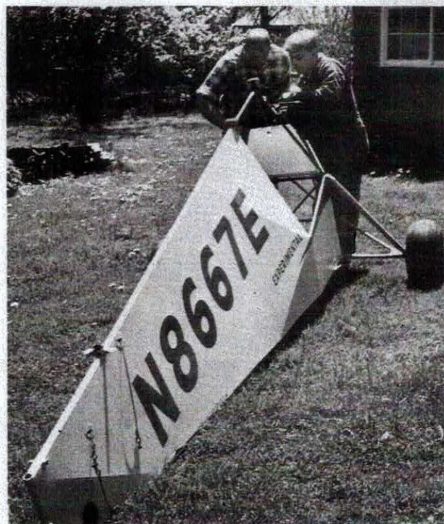
Fuselage of Headwind is simple triangular shape.
