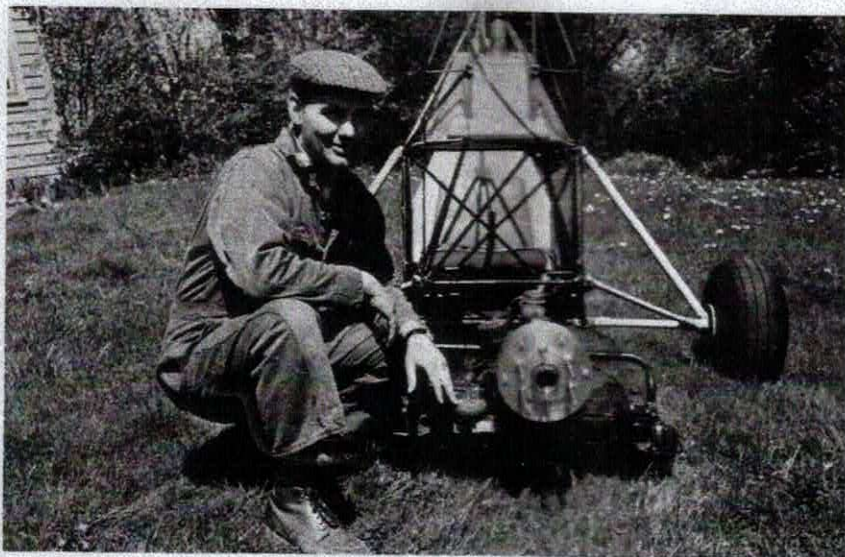
Don Stewart poses with VW engine, showing propeller reduction gear he designed.
