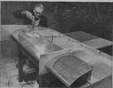
CALVIN PARKER drills rivet holes in leading edge of wing, which is held in place by plywood template
