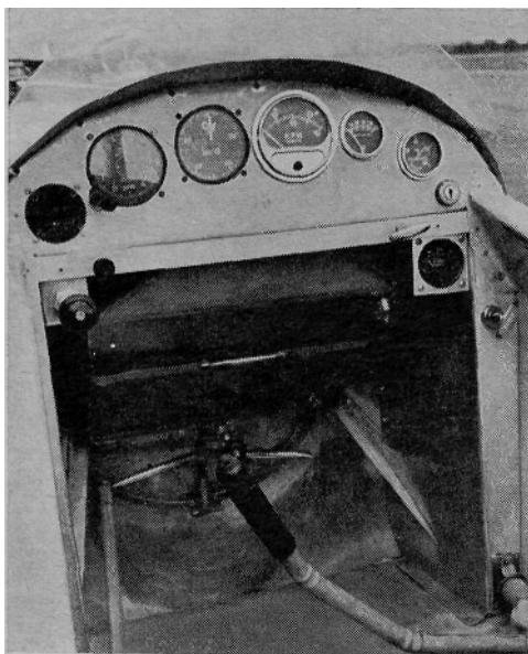
SIMPLE COCKPIT layout has basic instruments, off-set stick, rudder bar and push rods to controls
