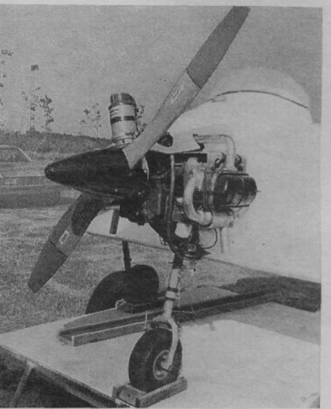
VOLKSWAGEN ENGINE was key around which plane was designed. Tricycle gear uses three go-kart wheels
