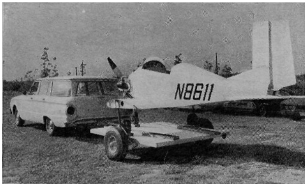
JEANIE'S TEENIE has removable wings which can be stowed in station wagon while the plane is towed
